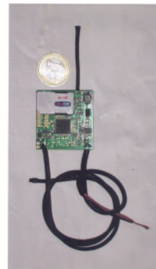
GSM Based Audio Eavesdropping Device discovered on a major Corporate Jet Aircraft at a major UK airport
